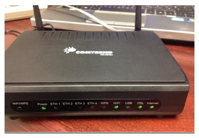
If your Geetel DSL modem is a black Comtrend AR-5312u or AR-5319 wireless modem/router combination, the lights across the front of the modem are as follows:
